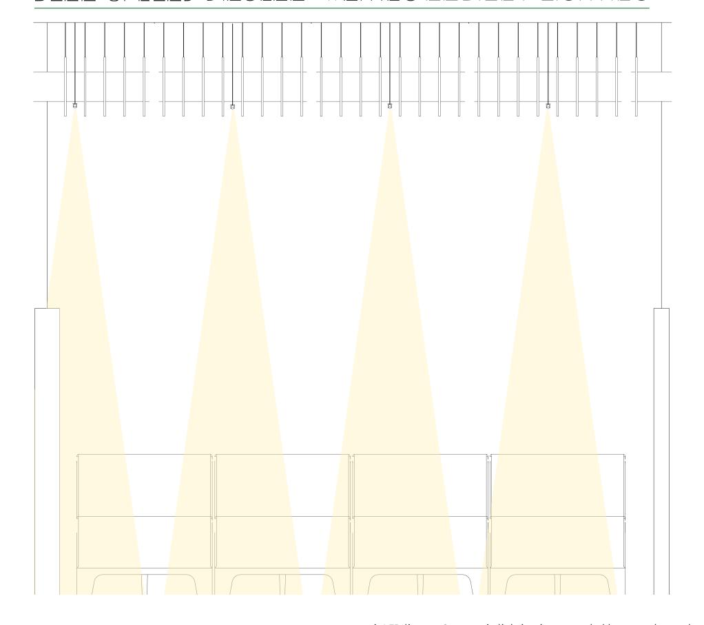
ioLED line .75 Symmetric lighting is suspended between layered acoustic blades to provide general ambient lighting to the waiting and host areas. The lights are dimmable to provide lower lighting levels.
