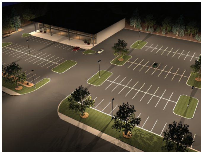
Prevail A40 LED 14 Fixtures = 2,002 Total watts
