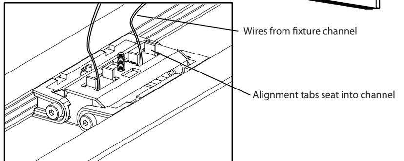
A. Run quick disconnects from fixture channel through top holes on panel yoke. Secure panel yoke with 1/4-20 bolt to fixture channel. Ensure tabs seat within fixture channel.
