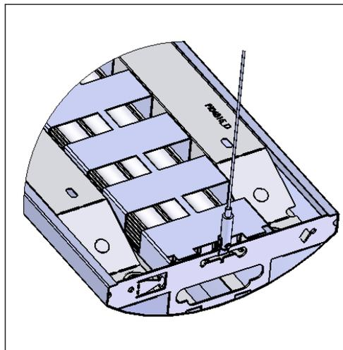
Remove film from optic before installing. To install - set in place over lamps. The Slide-N-Lock™ comes preset from the factory to the customer specified optical setting. To adjust, depress the control notch and slide tab to desired setting.
