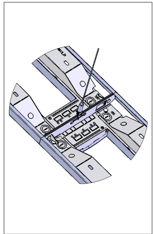
Tuck wires into wire cavity, slide both fixtures together and secure tightly using two 10-32 x 3/8" screws, starwashers and nuts. Tighten 1/4 turn past hand-tight. Starwashers must break the paint for proper grounding to occur.
