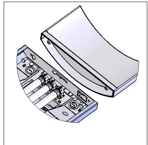
Align End Caps with end bracket of fixture. Secure using two 10-32 x 3/8" self-tapping screws.
