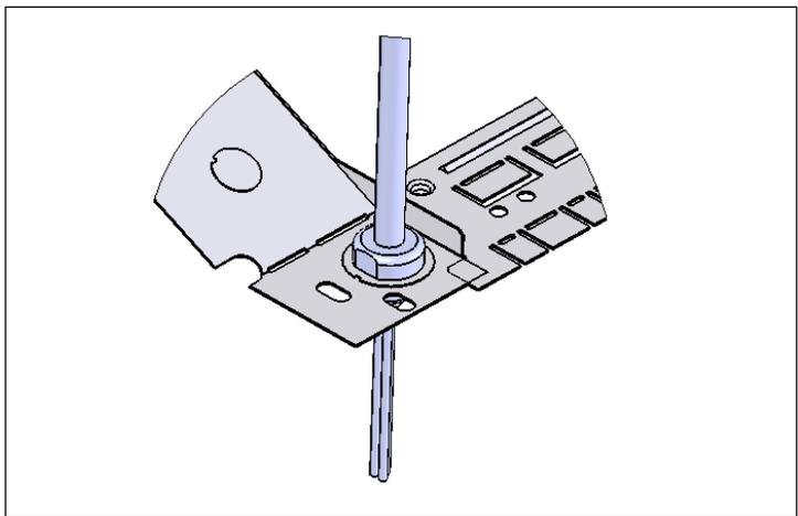
Break off appropriate KO, slide power cord through KO opening, then secure power cord with strain relief.
