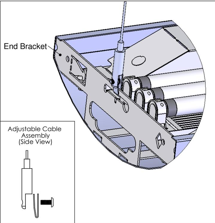
Slide adjuster clip into slot on end bracket. Secure machine screw to adjuster through the holes in the clip, tighten screw, but leave enough of a gap in the clip to slide back and forth. Slide cable through adjuster. Repeat on the opposite end for 1st fixture of row or stand-alone fixtures. For multiple fixtures, level 1st fixture, hang 2nd and level, etc. Level the complete row prior to tightening all the screws.
