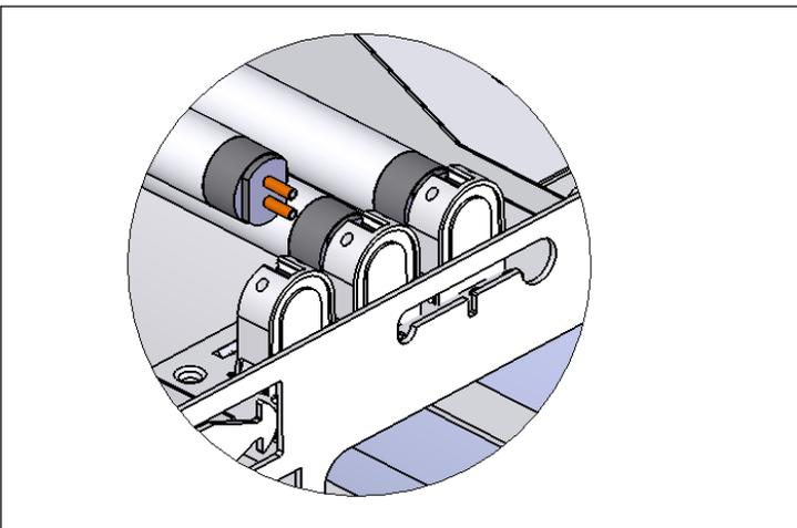
**NOTE:** Ensure lamps are properly seated before initial power-up. Push lamp down into socket and turn 90 degrees.
