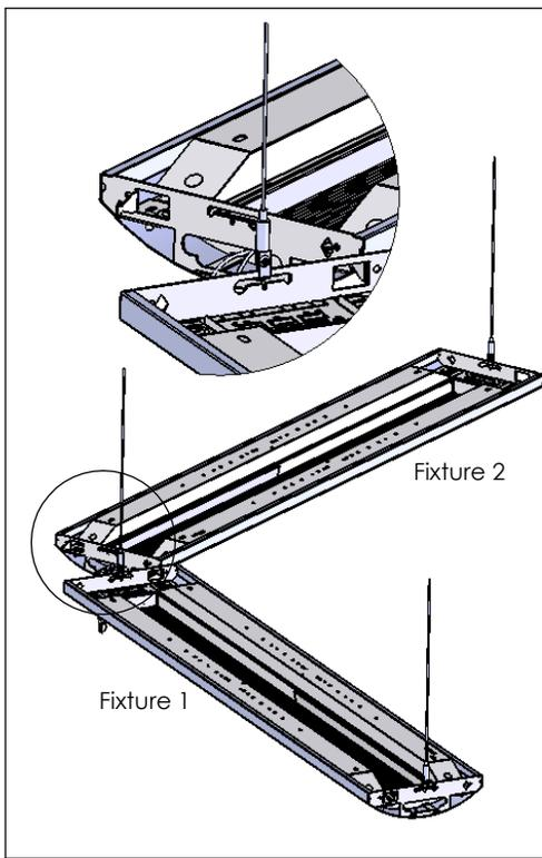
Install first fixture with two AC cables, then second fixture with one additional cable.
