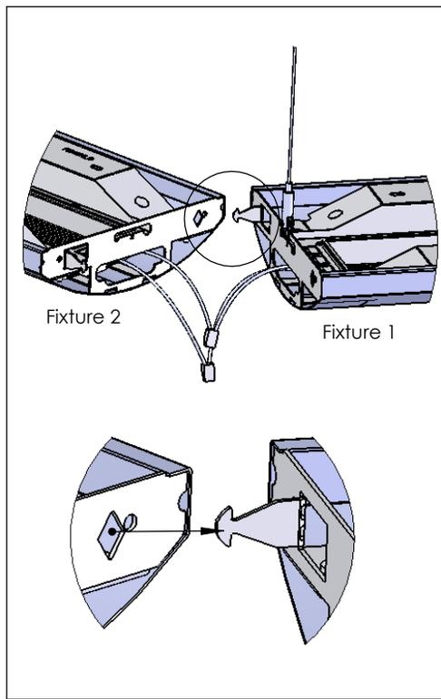
Bend out tapered aligning tabs and fit into aligner slots. (Fixture 2 is now supported by Fixture 1 at the joint.) Make electrical connections.
