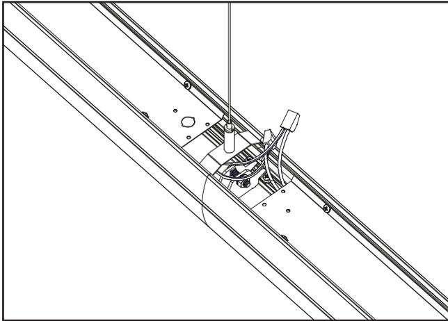
8. At lens joint, install lens cover.
