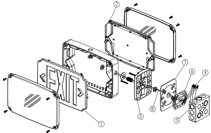
**On fixture with battery:** Connect battery only after continuous power can be supplied to fixture. Allow 24 hours before initial test or for full charge.
