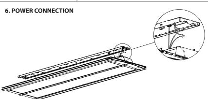
**A.** Make power connections between Fixture and J-Box following all National and Local Electrical Codes.
