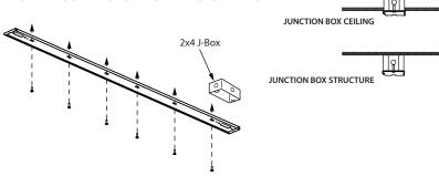
**A.** Starting with J-Box located at one end, fasten the MOUNTING BRACKET to ceiling/structure (hardware by others) using all mounting holes.
