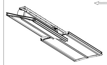
**B.** Once securely hooked, slide fixture away from neighboring fixture to create a gap sufficient enough to make through-wire connections.
