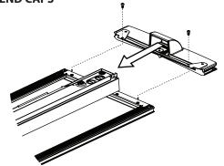
$\boldsymbol{\mathsf{A}}.$  Attach END CAP on FIRST and LAST fixture of continuous row.
