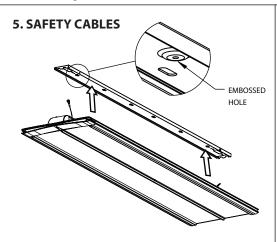
**A.** Attach SAFETY CABLES to SURFACE MOUNTING BRACKET using provided hardware at embossed holes (shown).
