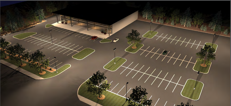
AFTER LED 14 Fixtures = 2,002 Total Watts
