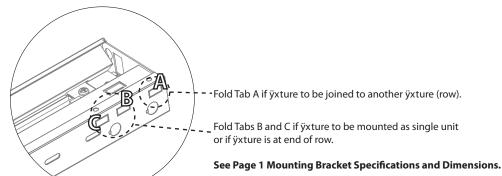
Hang Fixture on MOUNTING BRACKET and secure with included fasteners.
