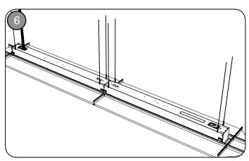
FOR CONTINUOUS RUNS: Secure next fixture in row using support wires on both sides of fixture. OPTIONAL STEP: Secure fixture to grid using #8 screws through grid bracket. Required for seismic installations. Repeat steps 5-6 as necessary.
