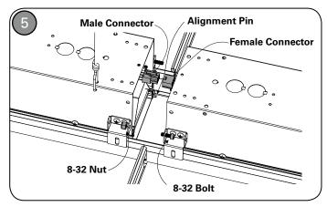
FOR CONTINUOUS RUNS: Connect through wiring using the provided push-in connectors, pressing together until they click into place. Tuck wiring into fixture and push together ensuring alignment pins are properly connected into mating features of the next fixture. Secure run using #8-32 bolts and nuts on each side of fixture through grid brackets.
