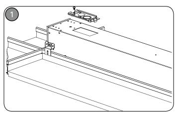
Prepare grid width spacing according to chart above and local building code. Install fixture housing into grid. Ensure Grid brackets secure over grid and fixture is resting on grid tee. Unscrew access plate and slide to remove as shown.
