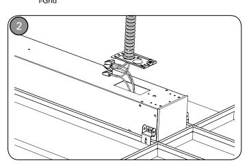
Connect shielded cable to access plate. Connect electrical wiring as required using provided push-in connector. Ensure wires are fully secure in connectors.
