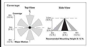
An optional integrated sensor system is available for maximum energy savings. A sensor is installed in each luminaire, turning the fixture on and off based on occupancy, and adjusting the fixture light output based on the amount of light around it (closed loop). The sensor system also acts as a control and programming input point to the system. See the DLVP system instruction sheet for more information.
