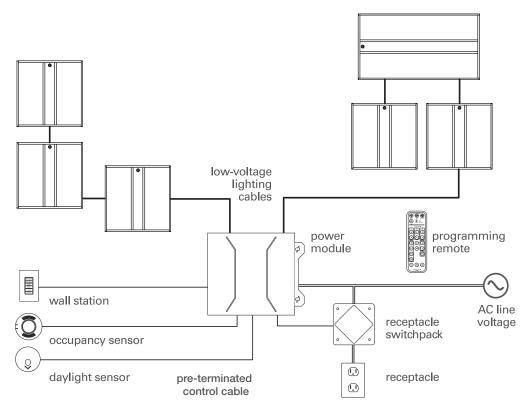
Note: When optional integrated sensors are used on any one zone, all luminaires on a power module must have integrated sensors. Optional integrated sensor shown.
