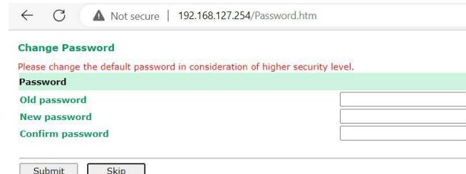
**Note:** (If you forget your password, the ONLY way to configure the NPort 6000 is by using the reset button to reset all settings and load the factory defaults. If you have disabled the reset button in your NPort 6000 configuration, you may still use it to load the factory defaults within the first 60 seconds that the NPort 6000 is powered on.)
