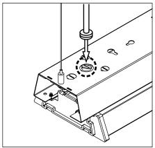
Break off appropriate knockout, slide power cord through KO opening, then secure power cord with strain relief.
