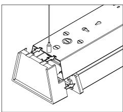
End Cap: Slide onto fixture end. Internal tabs to sit on top of flanges in spine and snap tabs will engage with top of fixtures.
