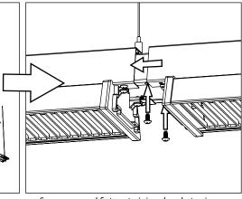
Secure second fixture to joiner bracket using two self-threading #10-32 screws. Fixture is now fully supported.
