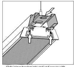
Slide joiner bracket into end and secure with two (2) self-threading #10-32 screws.
