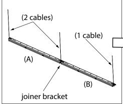
Install first fixture (A) with two aircraft cables, then second fixture (B) with one additional cable. Slide second fixture over joiner bracket.
