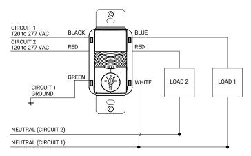
Three-way wiring diagram: Lights will turn OFF automatically when sensor that detected motion last, times out.
