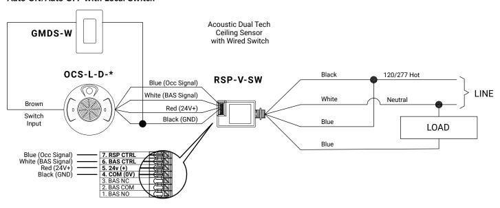
Note: Switchpack and the load switched by the switchpack MUST be fed from the same phase.
