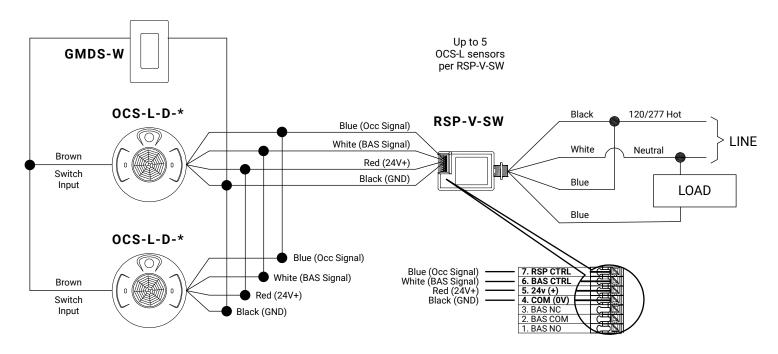
Note: Switchpack and the load switched by the switchpack MUST be fed from the same phase.
