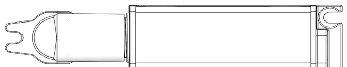
External Fixture Mounting with 90° Elbow (2 screws)
