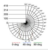
RA4LS9FSD2W1EWH-900Im-3000K Spacing criterion: (0-180) 1.15 | (90-270) 1.15 | (Diagonal) 1.22 Beam Angle: 89° Field Angle: 144° Lumens: 870 Input Watts: 8.7 W Efficacy: 100 LPW UGR: 20 Test Report: P710068
