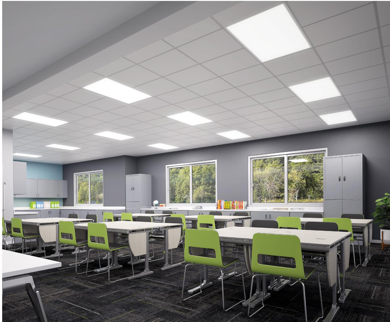
This edge lit selectable panel provides the high performance and aesthetic appeal of a flat panel while also providing the flexibility to adapt to the changing needs of a space, setting, or environment. Two large switches enable three selectable lumen levels (high, medium, low) and three selectable color temperatures (3000K, 3500K, and 4000K). FPS is an excellent lighting solution for commercial office spaces, schools, healthcare and retail merchandising areas.
