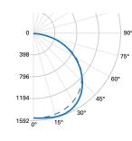
FILE NAME: DRI-WS-3L835-UNV-24-T1-STD.IES LAMP: (LD2) LED 3500K LUMENS: 5182 Lm WATTS: 40.3 W EFFICACY: 129 Lm/W TEST NO.: P189129 SC: (II) 1.35, ( $\perp$ ) 1.37 0° (II) \_\_\_\_\_
