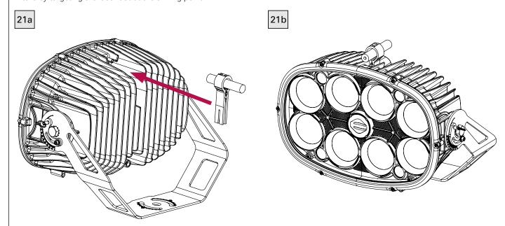
**Note**: Laser aiming may be difficult outdoors on bright sunny days. A diffuse reflective tarp located around the aiming point can facilitate aiming. The use of a daytime scope aimer is also available.
