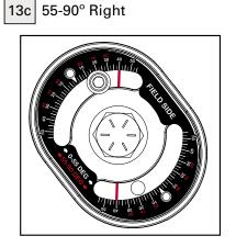
If laser aiming, tighten the mounting hardware so that fixture is secure but do not fully torque hardware until final aiming is complete. If using the orient gauge, torque the mounting hardware at this step to the values in the table below. If you are laser aiming, torque the hardware to the specification once the fixture is aimed.
