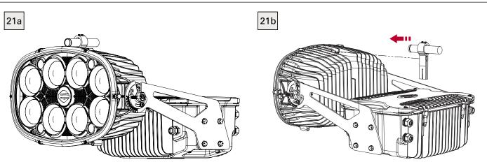
Turn on the laser and aim the fixture by targeting the laser dot at the aiming point.
