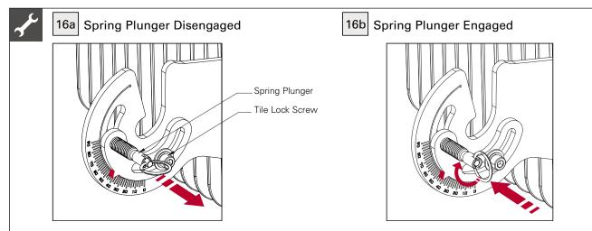
Rotate the labeled aiming plate until the arrow is over the desired tilt angle. Hold the aiming plate in place and tighten the tilt lock screw.
