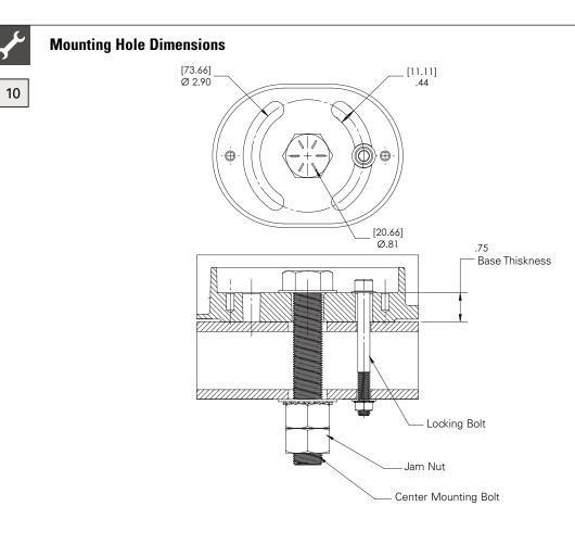
The Driver Box mounting hole is located underneath the orange cover on the base of the driver box. The central hole is sized for a <sup>3</sup>/<sub>4</sub>in bolt and the crescent shaped features are sized for a 3/8in bolt.
