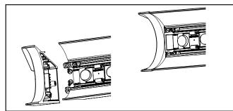
Re-install baffles. If required, use provided gaskets to ensure there is no light leak between each baffle section. (The bottom color of the gasket should match the color of the baffle). The baffles snap in and out of the fixture.
