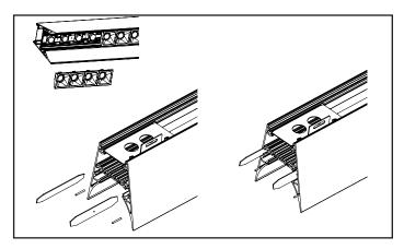
Hang the next fixture in the run on the Dual Bracket (E), attach the safety cable and make through wiring connections.
