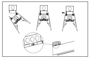
For next fixture, if fixture has baffles remove one baffle section at each end and secure Biscuit Aligners (G) half way into fixture end using hammer as needed. Install large end of Taper Pins (H) into fixture.
