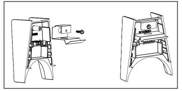
Slide End Cap onto the end of the fixture until the Spring Clip snaps onto the previously installed Spring Latch (K) in Step 2.
