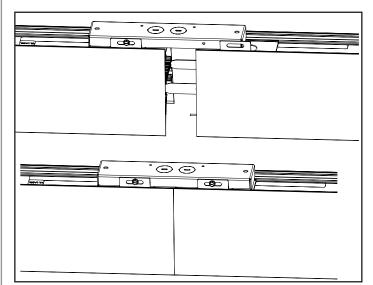
Once fixtures are together fasten together with Cast Joiners (C) and #8-18 x 1/2 HWH screws (B).
