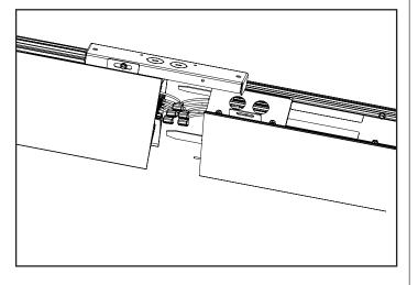
Tuck wiring into the inside of the fixtures, rotate the fixture up and push the two fixtures together. Secure with #8-18 x 1/2 HWH screw (B).
