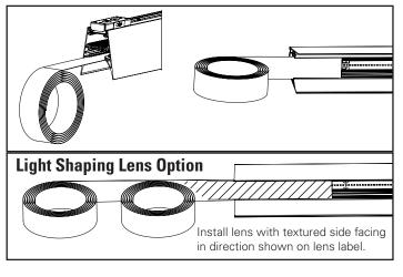
IMPORTANT: Ends of lenses should overhang fixture by ¼" at each end. Trim lens where necessary. **DO NOT UNDER-CUT.**
