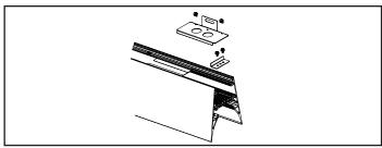
Align End Cap Spring Latch (K) to the end of the fixture as shown.
