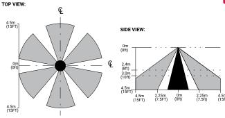
Note: Installation of integrated sensors within 3-ft (1m) of HVAC air vents is not recommended. The pattern shown is intended solely as a general quide and is not to scale.
