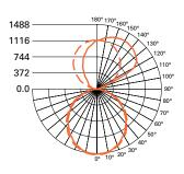
FILE NAME: SQW-F-075U-100D-835-1D-UNV-STD-W-4.IES CCT/CRI: 3500K / 80CRI LUMENS: 7116 Lm WATTS: 57.2 W EFFICACY: 124.4 Lm/W TEST NO.: P511798 43% UP / 57% DOWN 0° (II) \_\_\_\_\_\_ 0° 90° (⊥) \_\_\_\_\_\_
