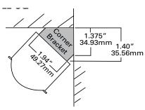
**HVSL2-SQ-X-WMAB45**=HVSL2-SQ Wall Mount Angle Bracket, 45 degree, specify length, (X=2,3,4,8)
