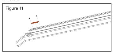
Secure both ends of the fixture using support wire through the grid brackets, according to local building codes (not supplied).
