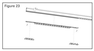
Reinstall LED trays. Reinstall Baffles.
