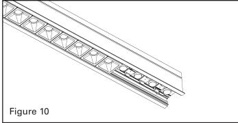
Remove access plate, make electrical connections, and reinstall.
