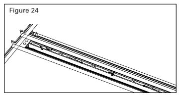
Slide lens film into the housing slot. If using a Perceive lens, install the perceive lens on the room side of the fixture. Install the lens with the textured side facing in the direction shown on the label.
