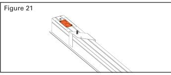
Install housing into ceiling using brackets, all-thread rods, or securing the housing directly to bracing.
