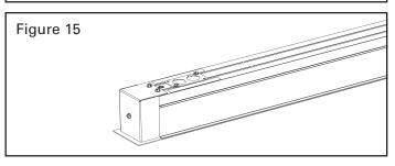
Removing the LED tray is required to secure the fixture in the ceiling. To do so, remove the baffles at both ends of the fixture, and in the center if 8ft.
