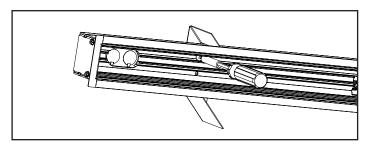
For continuous runs, make the electrical connections between the two fixtures. Then slide fixtures together, making sure the wires don't get pinched. Use cast joiners to secure the fixtures.
