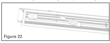
If using the drywall brackets, use a screwdriver to rotate the brackets into position behind the drywall. Tighten the screw to get the flange flush with the ceiling. Drywall brackets are designed to work with 1/2" and 5/8" drywall ceilings. Alternate thicknesses may require the use of a different screw.
