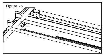
Place magnet into the end cap recess. Trim lens as necessary. Lens should extend 1/8" from each end of the housing extrusion.
