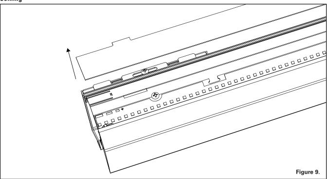
Remove dust cover from fixtures to access joiner aligner (Figure 9)
