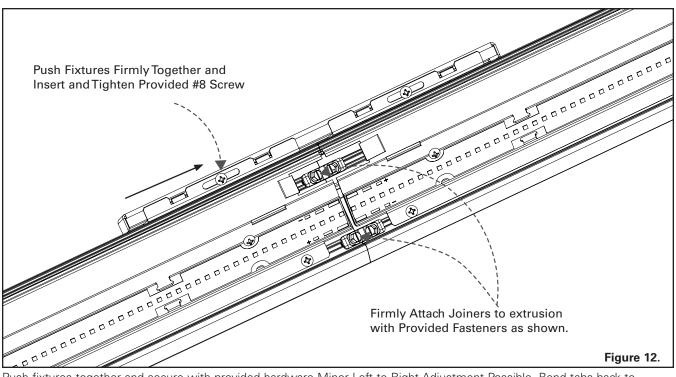
Push fixtures together and secure with provided hardware Minor Left to Right Adjustment Possible. Bend tabs back to original position (Figure 12.)
