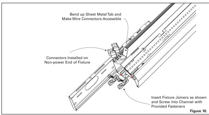
Bend up sheet metal tabs and pull wire and connectors up as shown. Insert and fasten the provided fixture joiners as shown (Figure 10.)
