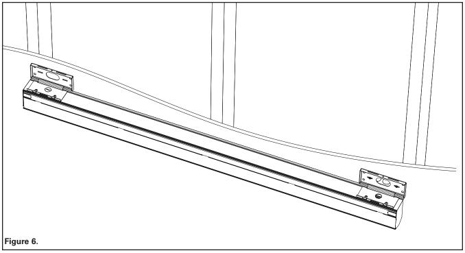
Hang first fixture from the installed brackets by hooking the flange on the fixture side bracket into the lower flange on the wall side bracket. Pull wires from the junction box and into the wiring hole on the fixture. Pull wires from fixture and supply wires out of the end of the fixture and attach using suitable connectors(by others) (figure 6,7, 8)
