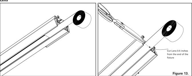
Insert the end of the roll in lens and push lens through the fixture run until it impacts the far end endcap. Cut the lens with sharp scissors a minimum of 0.5" past the end of the fixture. (Figure 13.)
