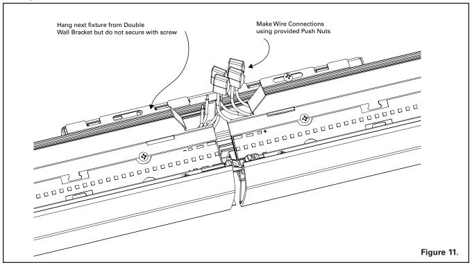
Connect wires using the provided wire connectors, push all wire back into fixture. (Figure 11.)
