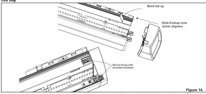
Attach joiners to the extrusion, slide decorative end cap onto joiners and fasten with provided hex head screws. (Figure 14.)
