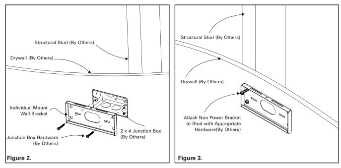
Mount subsequent wall brackets, level with the first, at the recommended spacing (See Table A) Brackets should be mounted to structure with appropriate hardware (by others)
