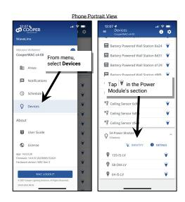
Note: Use the **Identify** button on the Low-Voltage Power Module to **reverse identify** the device in the **Devices** tab. When the **Identify** button is pressed, the icon in the Mobile App **Devices** list will appear to pulse for 15 seconds.
