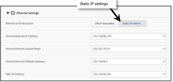
If changes were made, click on **SAVE** and then close the web browser. The Low-Voltage Power Module will automatically reboot once Ethernet setting changes are saved. If the web browser has been left open, it will be disconnected. A Low-Voltage Power Module reboot takes approximately 1 ½ minutes to complete.
