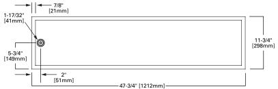
Shown with either Sensor OR Integrated Emergency test switch. For units with both Emergency and Sensor there is one holder on each end.
