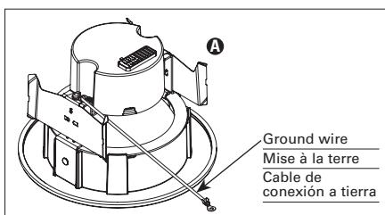
2. Connect other end of ground wire to housing. Connection to housing may vary depending on model. Three connection methods are described below.
