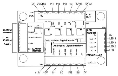
iCANnet cable type - Cooper LC Cable or Belden™ 1502R (NON PLENUM) or 1502P (PLENUM) 100 Devices per physical segment on iCANnet (BN-2-NA can be added to combine more than 100 devices together, up to 65,000 total)
