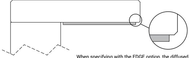
When specifying with the EDGE option, the diffused glass becomes thicker adding a visible line of light around the edge accentuating the luminaires' aesthetics and styling.
