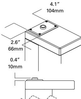
Photocontrol cover is precision machined from corrosion-resistant 6061-T6 aluminum and is secured to bollard head with tamper resistant stainless steel hardware. The photocontrol option is available in dedicated 120V or 208-277V. When specifying a photocontrol option make sure to designate the appropriate voltage within the catalog logic.
