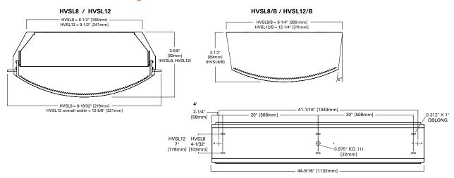
(8' unit cnsists of (2) 4' units, attached at the factory)
