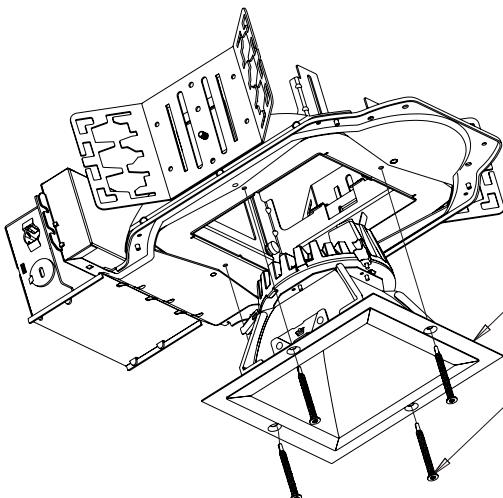
Antimicrobial powder coated security plate attached to the reflector flange with mechanical tabs and high strength adhesive.
