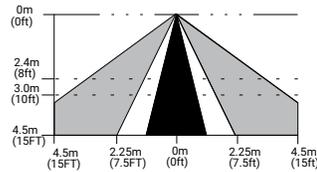
**Note:** Installation of integrated sensors within 3-ft (1m) of HVAC air vents is not recommended. The pattern shown is intended solely as a general guide and is not to scale.
