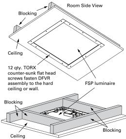
Position the DFVR assembly in the ceiling cut-out, and secure with multiple tamper-resistant screws; shown above.
