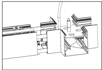
Bend up tabs to expose the tops of the cast joiner screws.
