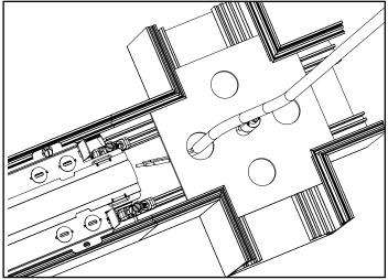
Pull the 5 wire connectors out of the opening of the next fixture in the sequence for ease of wiring.
