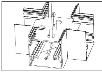
The cover plate can be temporarily hung from the SJ cord, using the provided strain relief, if the SJ is already attached to the canopy.
