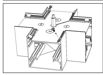
Insert the SJ cable through the hole as shown below. (Strip the main jacket to expose at least 8 inches of loose wire).
