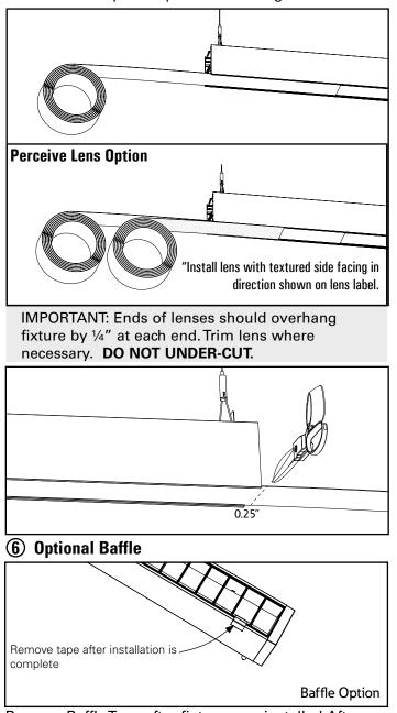
Remove Baffle Tape after fixtures are installed.After removing tape, take care to ensure that the down-light baffle components are spaced appropriately so that there is minimal gap between them.
