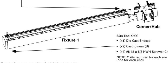
For installation at ceiling, see separate ceiling interface instructions.
