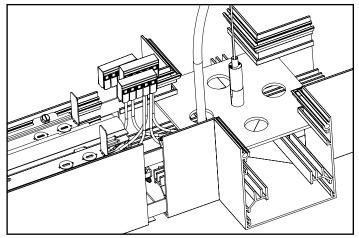
Slide the fixtures together and drive the provided #8-18 by 1/2" screws into the hub/corner as shown.
