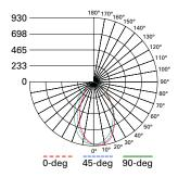
LCR412WW9FSE020-12W-3000K Spacing criterion: (0-180) 0.91 | (90-270) 0.98 | (Diagonal) 1.01 Lumens: 1255 Input Watts: 12.1 W Efficacy: 103.7 LPW Test Report: P645618
