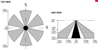
Note: Installation of integrated sensors within 3-ft (1m) of HVAC air vents is not recommended. The pattern shown is intended solely as a general guide and is not to scale.
