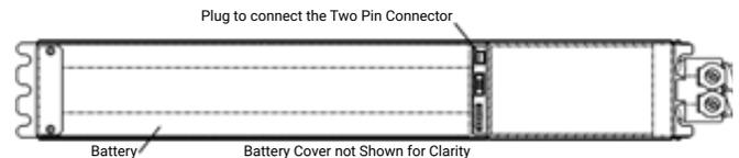
6. Replace the old battery and connect to the two-pin connector which comes from the wire of the new battery to the existing two-pin connector plug.
