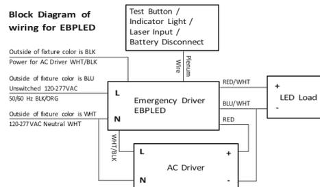
The unswitched AC power for the EBP and the power for the AC driver should be from the same branch circuit to prevent disconnecting two (2) sources of power and the battery during servicing. Key and store it for later use..
