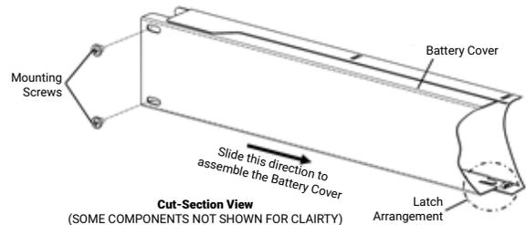
8. Install the EBP back using the necessary hardware.
