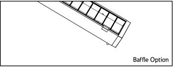
After fixtures are installed, remove baffle tape. Take care to ensure the downlight baffle components are spaced appropriately so that there is minimal gap between them.
