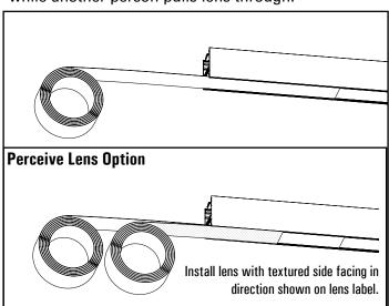
IMPORTANT: Ends of lenses should overhang fixture by ¼" at each end. Trim lens where necessary. **DO NOT UNDER-CUT.**
