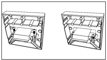
Slide end cap onto the end of the fixture until the snap engages.
