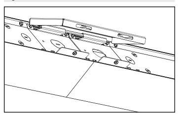
Rotate fixture until level and secure with the provided  $\#8-18 \times 3/8$  HWH screws.
