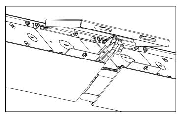
Tuck wiring into the inside of the fixtures and push the fixtures together.
