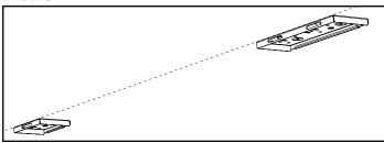
Hang fixture from brackets as shown below and secure safety cable to the surface mount bracket.
