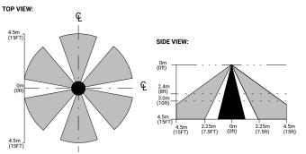
Note: Installation of integrated sensors within 3-ft (1m) of HVAC air vents is not recommended. The pattern shown is intended solely as a general guide and is
