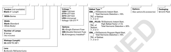
NOTES: (1) Products also available in non-US voltages and frequencies for international markets. (2) Not available when specifying emergencies, voltage must be specific. (3) Stem mounting not available on 3-lamp fixtures. (4) 2 point suspension recommended for 2 and 4-lamp fixtures. (5) Steel endplates with 7/8" KO standard for continuous row mounting. (6) Please specify required voltage, 120V or 277V.
