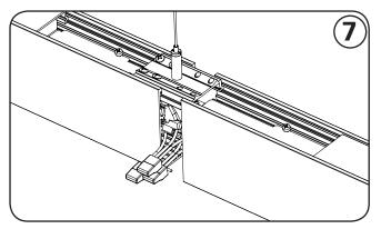
FOR CONTINUOUS ROWS ONLY: Hang far end of the next fixture in the row using the griplock® and pre-installed aircraft cable. Temporarily rest adjoining fixture on the first and join dimming and power wires using the provided push nuts.
