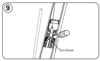
While one person holds fixtures in place check to make sure fixture is level. DO NOT WALK AWAY LEAVING THE FIXTURES UNFASTENED BY MECHANICAL MEANS. Fixture can be leveled via grip lock on opposite end of fixture. Once fixtures are flush to one another and level install torx head screw through cast joiners to snug fixtures together. DO NOT OVER TIGHTEN. Torx screw will pull fixtures together tightly without too much force.
