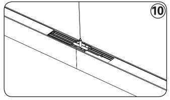
Replace all access plates and move lenses back to proper positions. The fixture installation is now complete
