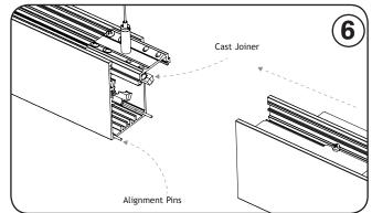
FOR CONTINUOUS ROWS ONLY: Hang far end of the next fixture in the row using the griplock® and pre-installed aircraft cable. Temporarily support the other end. Ensure the alignment pins and cast joiners are seated correctly in the adjoining fixture
