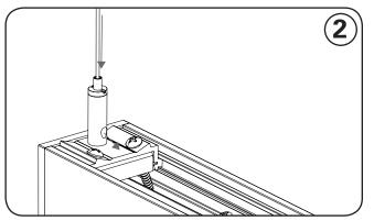
Pull aircraft cable through griplocks® and adjust to desired height. Make sure to level the fixture correctly (applies to individuals or first piece in row).
