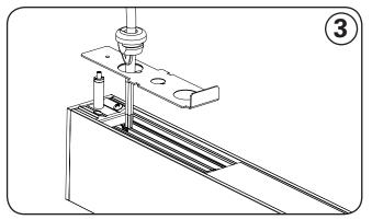
Remove knockout from access plate and attach strain relief to SJ Cord .Pull SJ cord through access plate to lock SJ cord in place on access plate.
