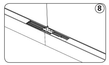
Slide fixtures together ensuring that both fixtures are level and properly aligned.
