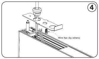
Connect power and dimming leads to SJ cord as required using wire nuts (by others) Once power and dimming wires are connected, push the wiring back into the fixture and re-attach the access plate.
