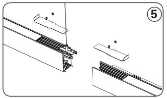
Remove non-wiring access plates from both fixtures prior to joining by removing two #8-32 screws. (Fixture information and UL labels should be visible on both sides of the non-wiring access plates
