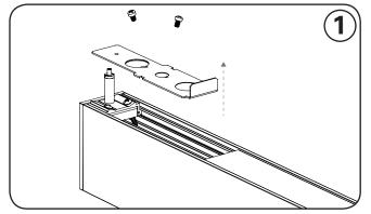
Turn off power before installation. Connect mounting kits at pre-specified locations according to your specific ceiling type (see submittal for dimensional details). Remove fixture from box and remove access plate by slidinng the lens out of the way andremoving two #8-32 screws.
