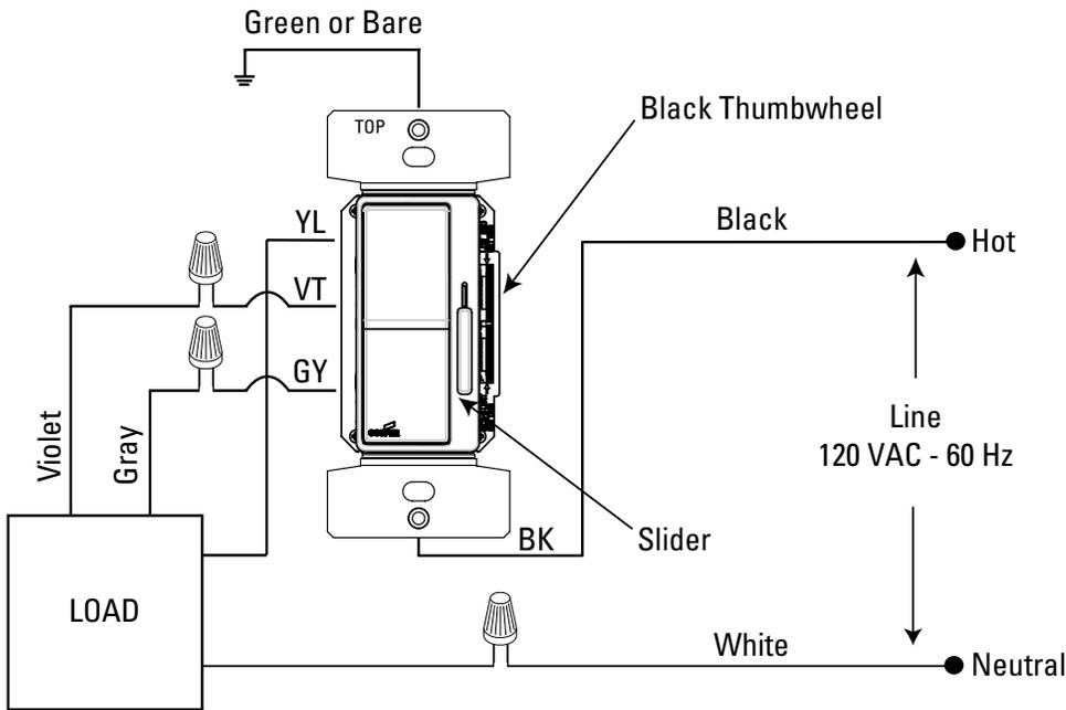
**FIGURE 2: 3-WAY WIRING DIAGRAM**
