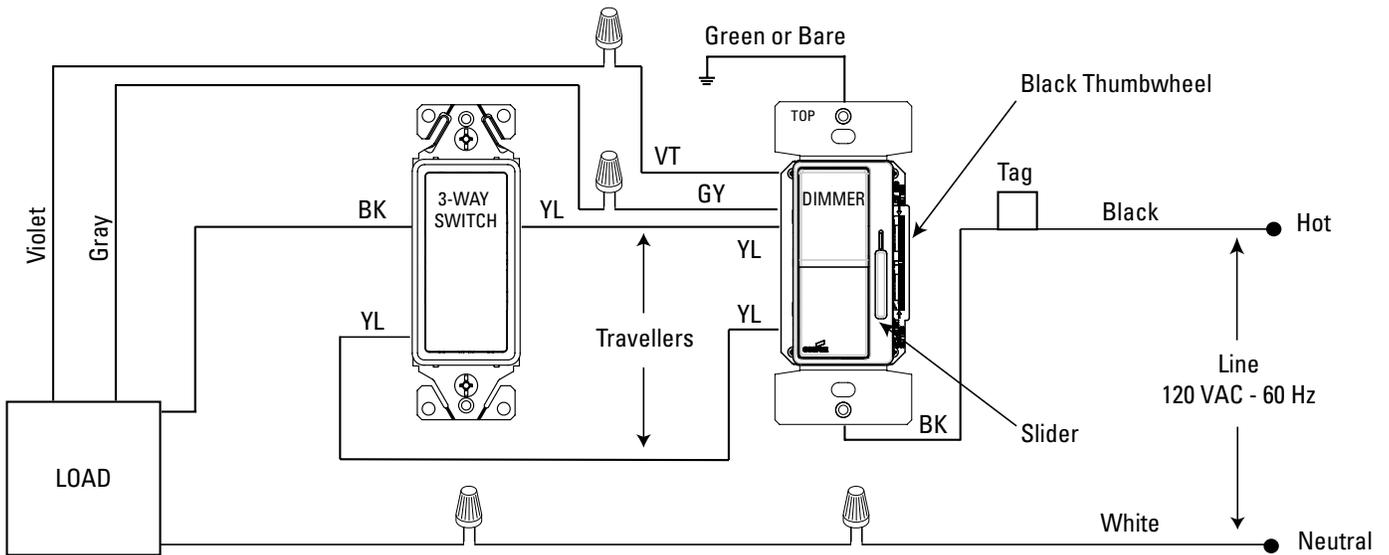
\*Can be installed on load or line side in 3-way applications
